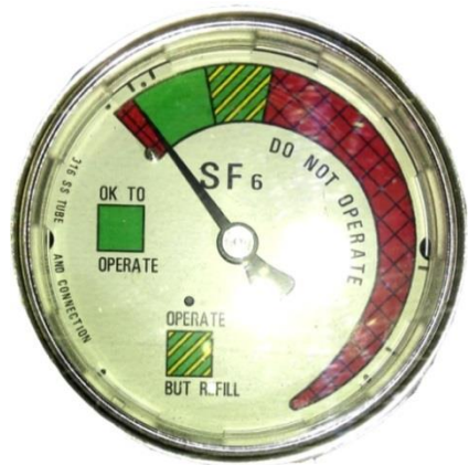
Figure B2. Old SF6 Gauge. Used on switches purchased before 2011.
