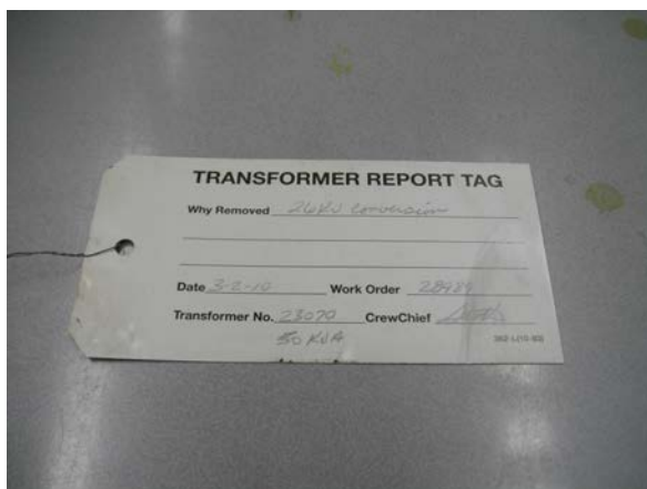
Figure 4.2. Transformer Report Tag
