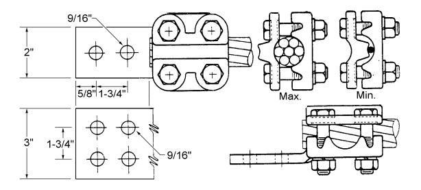
**Terminal Connector Lugs** of the Universal type shall be of the general configuration shown and shall be forged or cast from high-conductivity copper alloy. The bolts, nuts, and lock washers shall be high-strength silicon bronze. The connectors shall meet the applicable requirements of ANSI/NEMA CC-1, *Electric Power Connectors for Substations*.
