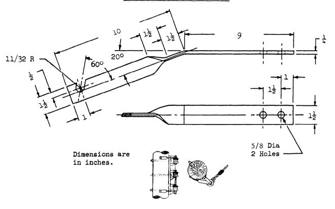
SECONDARY RACK REINFORCING STRAPS shall be of the configuration and dimensions shown, and shall be made of hot-rolled bar steel conforming to ASTM specification A 107.
